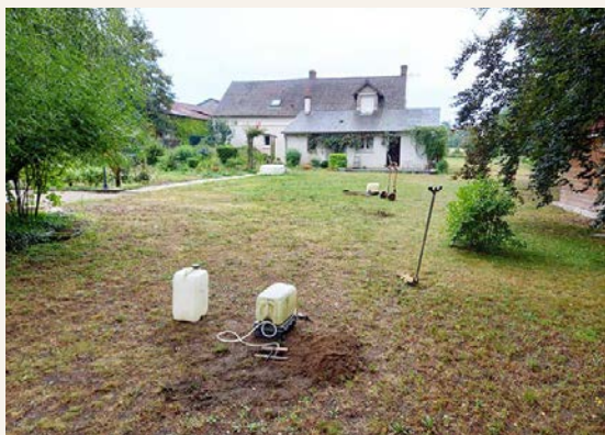
Test de type porchet (source HYDRO41)
